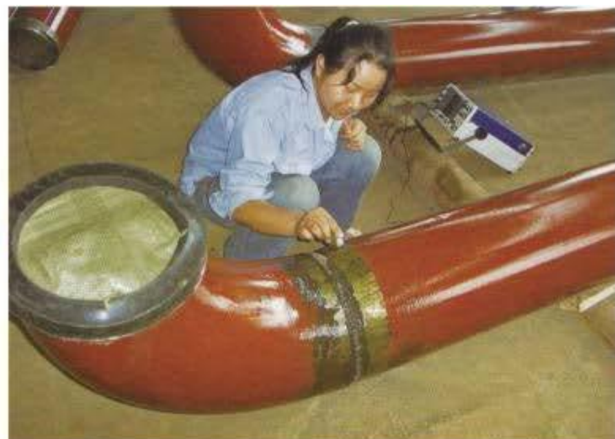
焊缝探伤 (Infiltration detection)
